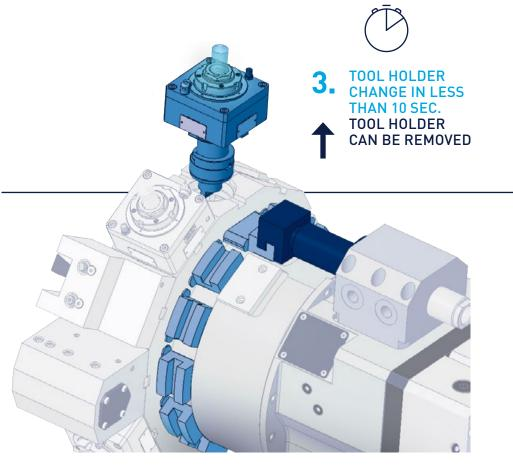
The QUICK-LOCK BMT® tool holder system is based on the worldfamous EPPINGER BMT interface. A simplified access to the change station is always given. Several turrets can be equipped easily by the same external location.
